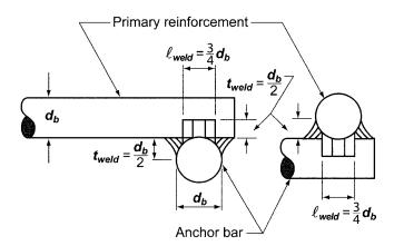
Fig. R16.5.6.3b—Weld details used in tests of Mattock et al. (1976a).
