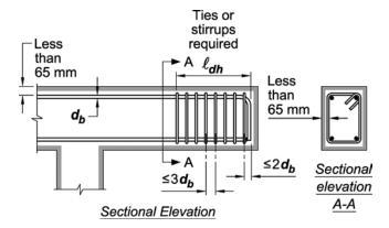
Fig. R25.4.3.3—Concrete cover according to 25.4.3.3.
