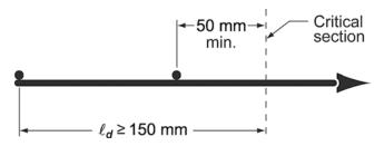
Fig. R25.4.7.2—Development of welded plain wire reinforcement.
