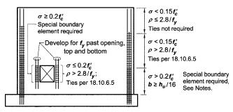
Notes: Requirement for special boundary element is triggered if maximum extreme fiber compressive stress  $\sigma \geq 0.2f_{c}'$ . Once triggered, the special boundary element extends until  $\sigma < 0.15f_{c}'$ . Since  $h_{w}/\ell_{w} \leq 2.0$ , 18.10.6.4(c) does not apply.
