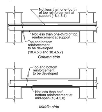
Fig. R18.4.5.3—Arrangement of reinforcement in slabs.
