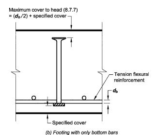
Fig. R20.6.1.3.5—Concrete cover requirements for headed shear stud reinforcement.
