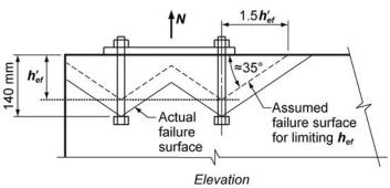
The actual  $h_{ef}$  = 140 mm but three edges are  $\leq 1.5 h_{ef}$  therefore the limiting value of  $h_{ef}$  (shown as  $h'_{ef}$  in the figure) is the larger of  $c_{a,max}/1.5 \epsilon$  d one-third of the maximum spacing for an anchor group:
