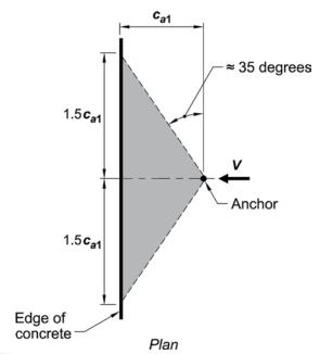
Fig. R17.3.2b—Breakout cone for shear.
