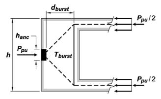
(b) Flanged section with end diaphragm
