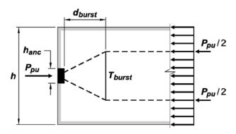
(a) <u>Rectangular section</u> T<sub>burst</sub> ≈ 0.25**P**<sub>pu</sub>
