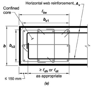
Option with standard hooks or headed reinforcement
