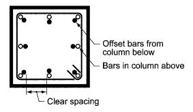
Fig. R10.7.5.1.3—Offset column bars.
