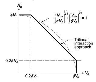
Fig. R17.6—Shear and tensile load interaction equation.
