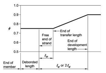
Note: The location of the end of development length depends on the calculated stresses in the extreme concrete fiber of the precompressed tension zone under service loads.
