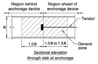
Fig. R25.9.1.1b—General zone for anchorage device located away from the end of a member.
