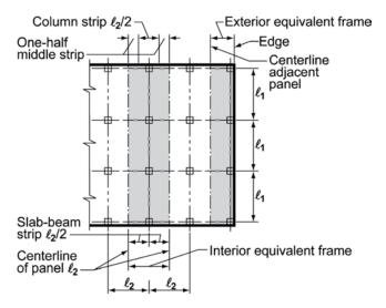
Fig. R8.11.2—Definitions of equivalent frame.
