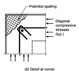
Fig. R25.7.1.6—Spalling of corners of beams subjected to torsion.
