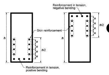
**Fig. R9.7.2.3**—Skin reinforcement for beams and joists with h > 900 mm.
