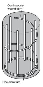
Fig. R25.7.2.3b—Continuous tie anchorage.
