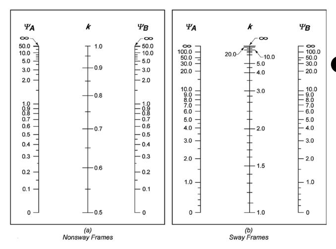
$\Psi$  = ratio of  $\Sigma(EII\ell_c)$  of columns to  $\Sigma(EII\ell)$  of beams in a plane at one end of a column
