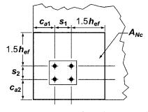
$A_{Nc} = (c_{a1} + s_1 + 1.5h_{ef})(c_{a2} + s_2 + 1.5h_{ef})$  if  $c_{a1}$  and  $c_{a2} < 1.5h_{ef}$  and  $s_1$  and  $s_2 < 3h_{ef}$
