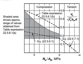
Fig. R22.5.6.1—Comparison of shear strength equations for members subject to axial force.
