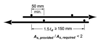
Fig. R25.5.4.1—Lap splices of plain welded wire reinforcement where  $A_{s,\,provided}/A_{s,\,required} < 2$ .
