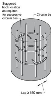
Fig. R25.7.2.4—Circular tie anchorage.
