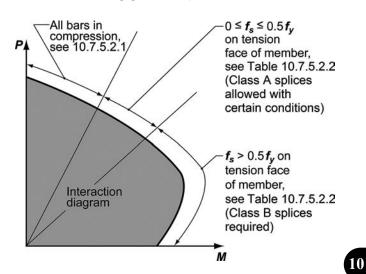
Fig. R10.7.5.2—Lap splice requirements for columns.
