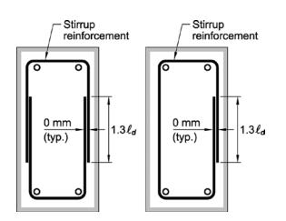
Fig. R25.7.1.7—Closed stirrup configurations.
