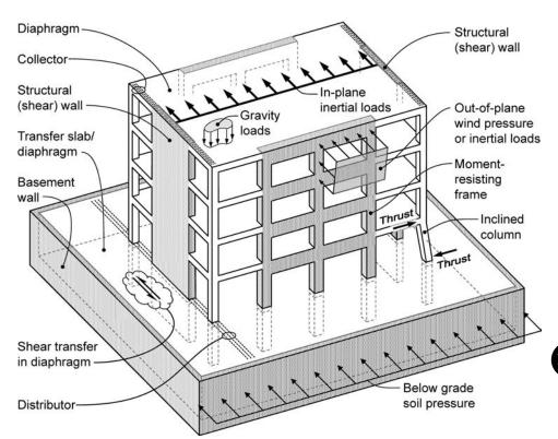
Fig. R12.1.1—Typical diaphragm actions.
