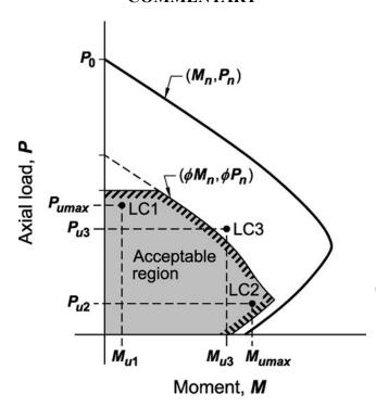
Fig. R10.4.2.1—Critical column load combination.
