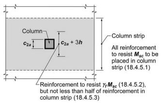
Note: Applies to both top and bottom reinforcement
