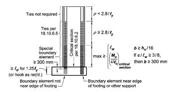
(a) Wall with  $h_W \ell_W \ge 2.0$  and a single critical section controlled by flexure and axial load designed using 18.10.6.2, 18.10.6.4, and 18.10.6.5
