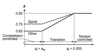
*Fig. R21.2.2b*—Variation of  $\phi$  with net tensile strain in extreme tension reinforcement,  $\varepsilon_t$ .
