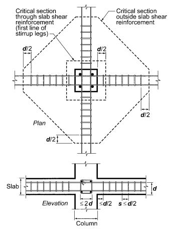
Fig.R8.7.6d—Arrangement of stirrup shear reinforcement, interior column.
