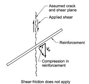
Fig. R22.9.4.3b—Compression in reinforcement.
