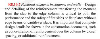
**R8.10.7.2** Equation (8.10.7.2) refers to two adjoining spans, with one span longer than the other, and with full dead load plus one-half live load applied on the longer span and only dead load applied on the shorter span.
