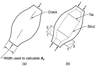
Fig. R23.4.3—Bottle-shaped strut: (a) cracking of a bottle-shaped strut; and (b) strut-and-tie model of a bottle-shaped strut.
