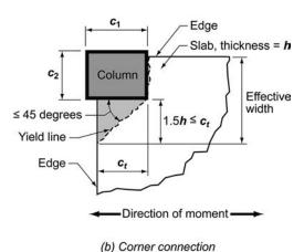
Fig. R18.4.5.1—Effective width for reinforcement placement in edge and corner connections.
