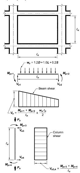
Fig. R18.6.5—Design shears for beams and columns.
