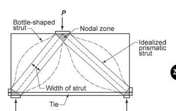
Fig. R23.2.1—Description of strut-and-tie model.
