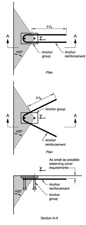
Fig. R17.5.2.9a—Hairpin anchor reinforcement for shear.
