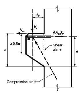
Fig. R16.5.1a—Structural action of a corbel.
