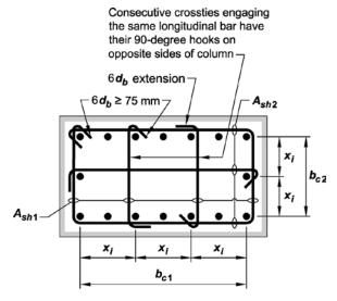
The dimension  $x_i$  from centerline to centerline of laterally supported longitudinal bars is not to exceed 350 mm. The term  $h_x$  used in Eq. (18.7.5.3) is taken as the largest value of  $x_i$ .
