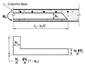
Fig. R22.6.9.6—Idealized shear acting on shearhead.
