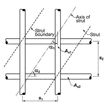
Fig. R23.5.3—Reinforcement crossing a strut.
