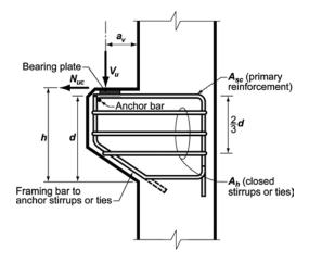
Fig. R16.5.1b—Notation used in Section 18.3.
