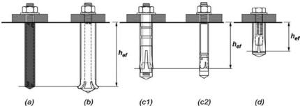
(B) Post-installed anchors: (a) adhesive anchor; (b) undercut anchor;(c) torque-controlled expansion anchors ((c1) sleeve-type and (c2) stud-type);and (d) drop-in type displacement-controlled expansion anchor.
