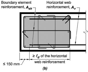
Option with straight developed reinforcement
