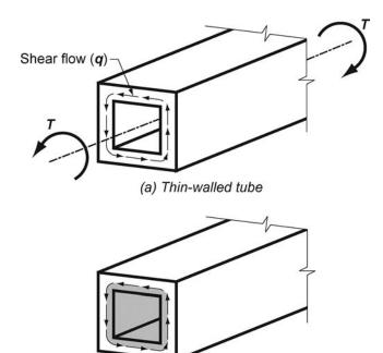
Fig. R22.7—(a) Thin-walled tube; and (b) area enclosed by
