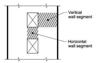
Fig. R18.10.4.5—Wall with openings.
