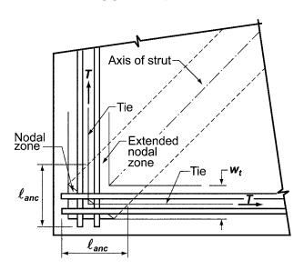
Fig. R23.8.2—Extended nodal zone anchoring two ties.
