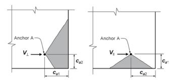
Fig. R17.5.2.1d—Shear force near a corner.
