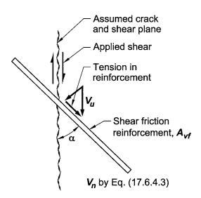
Fig. R22.9.4.3a—Tension in shear friction reinforcement.
