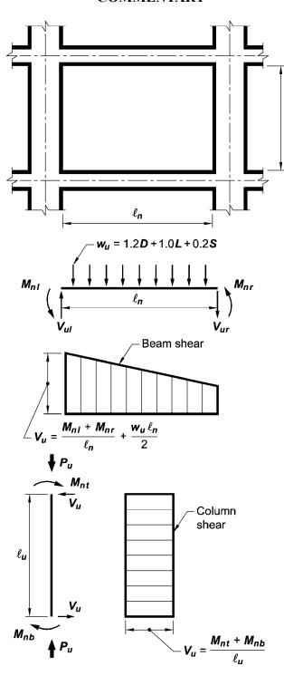
Fig. R18.4.2—Design shears for intermediate moment frames.
