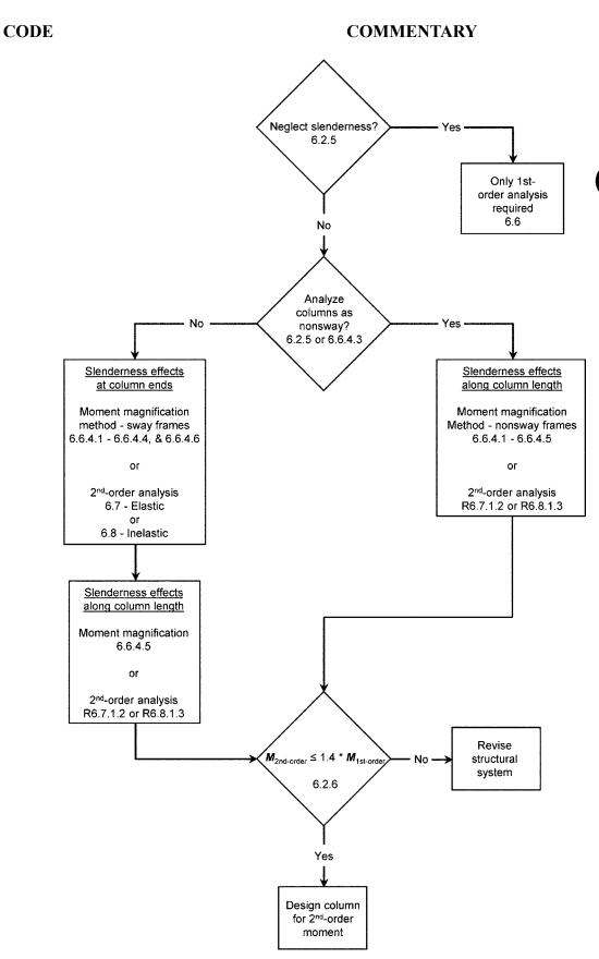
Fig. R6.2.6—Flowchart for determining column slenderness effects.
