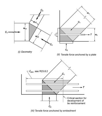
Fig. R23.2.6a—Hydrostatic nodes.
