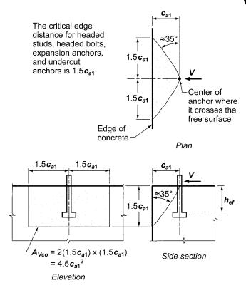
Fig. R17.5.2.1a—Calculation of A<sub>Vco</sub>.
