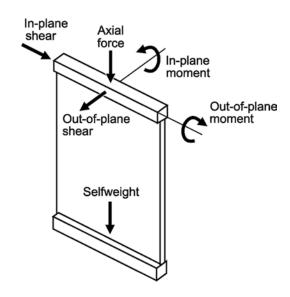
Fig. R11.4.1.3—In-plane and out-of-plane forces.
