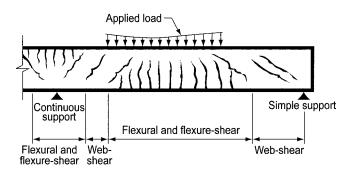
*Fig. R22.5.8.3*—*Types of cracking in concrete beams.*
