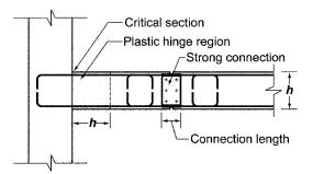
(a) Beam-to-beam connection
