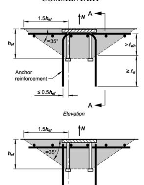
Fig. R17.4.2.9—Anchor reinforcement for tension.
