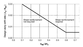
Fig. R18.14.5.1—Illustration of the criterion of 18.14.5.1.
