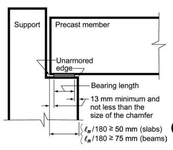
Fig. R16.2.6—Bearing length on support.
