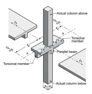
Fig. R8.11.4—Equivalent column (column plus torsional members).
