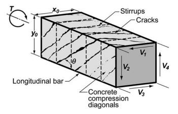
Fig. R22.7.6.1a—Space truss analogy.
