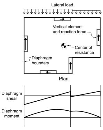
Fig. R12.4.2.3b—Diaphragm in-plane actions obtained by modeling the diaphragm as a horizontal rigid beam on flexible supports.
