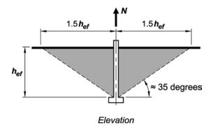
Fig. R17.3.2a—Breakout cone for tension.
