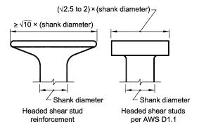
*Fig. R20.5.1*—Configurations of stud heads.
