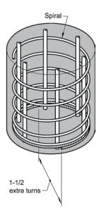
Fig. R25.7.3.4—Spiral anchorage.
